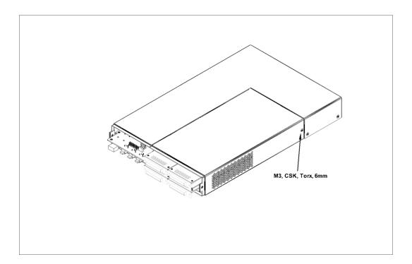
4. Slide off the function card cover in the direction shown:
