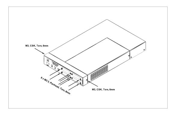
2. Carefully slide off the front bezel in the direction shown:
