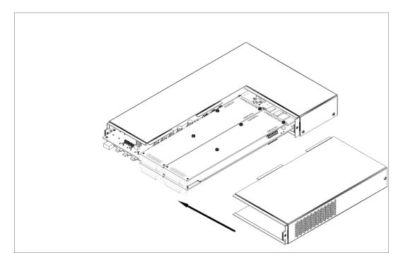
Make sure that the lips are positioned correctly underneath its counterpart. Check also the alignment on the bottom.
