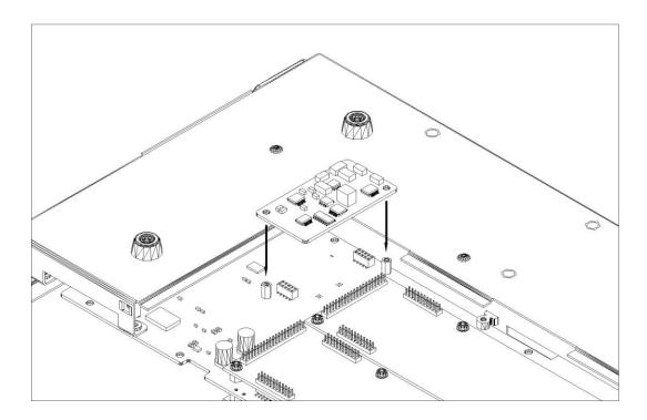
10. Attach it using two M2.5x6mm panhead screws and two M2.5 washers (delivered with the ProDAQ 3202):
