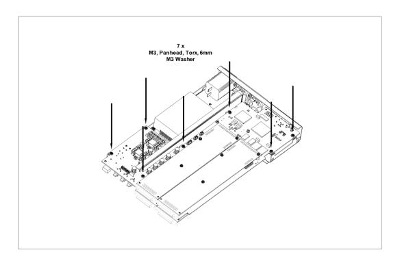
8. Now turn the whole chassis plus assembly over and slide the PCB assembly forward by about 30mm (1 1/5 inches). Be careful not to damage the tracks or parts while doing so. You may have to unplug one side of the cable connecting the power supply with the PCB or the fan cables:
