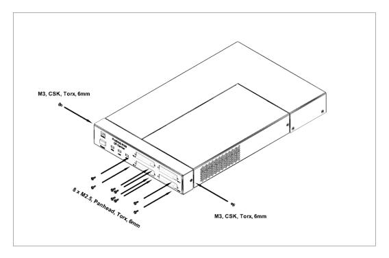
Then attach the function cards again to the front bezel using the eight M2.5x6mm panhead screws removed in step 1. The function cards are slightly flexible, so most likely the threaded holes of the connectors don't line up perfectly with the mounting holes in the front bezel. Don't force the screws into the threads, position the function cards correctly behind the front bezel first!
