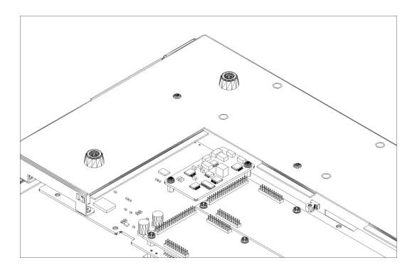
12. Turn the unit back over and slide the PCB assembly back into place. Avoid again scratching any tracks or damaging any parts while doing so.
